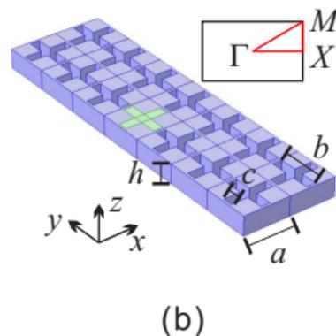
**Figure:** Phononic crystal slab of cross holes in stainless steel. The parameters  $b/a=0.9$ ,  $c/a=0.2$  and  $h/a=0.4$ , with the lattice constant  $a=20$  mm optimize the band gap width [49].
