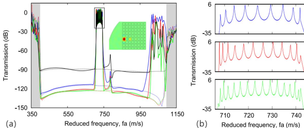
**Figure:** Channeled spectrum: sequence of frequency maxima and minima in the transmission spectrum. It depends mostly on the waveguide length.
