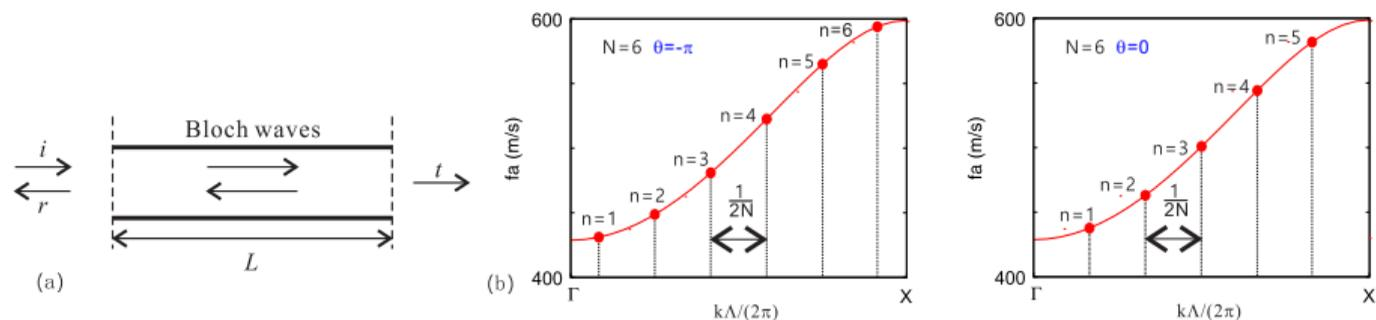
**Figure:** (a) Simplified model of transmission through a single-mode periodic waveguide at a single frequency. (b) Graphical construction of the channeled spectrum from the dispersion relation of the infinite waveguide.
