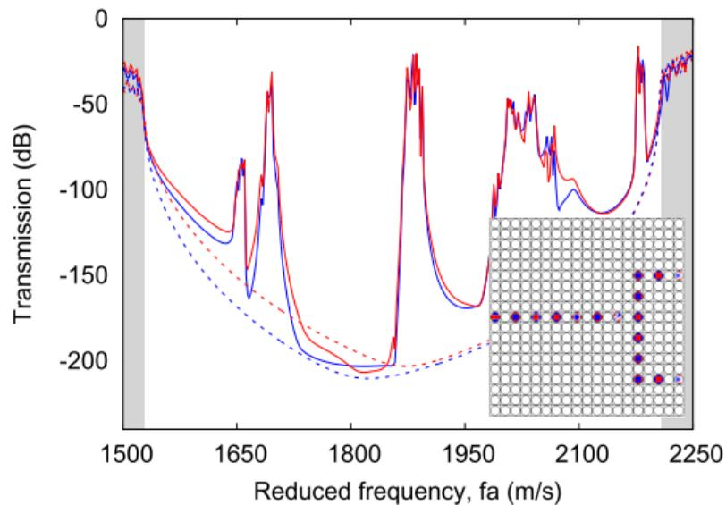
Figure: Splitter circuit: the symmetry of the Bloch wave allows for even splitting.
