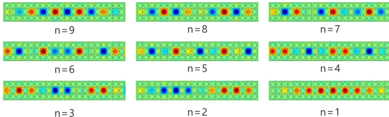
**Figure:** Pressure distribution of the straight CRAW (CW1,  $L = 10\lambda$ ) at the resonance peaks. The number of pressure oscillations is shown below the field maps.
