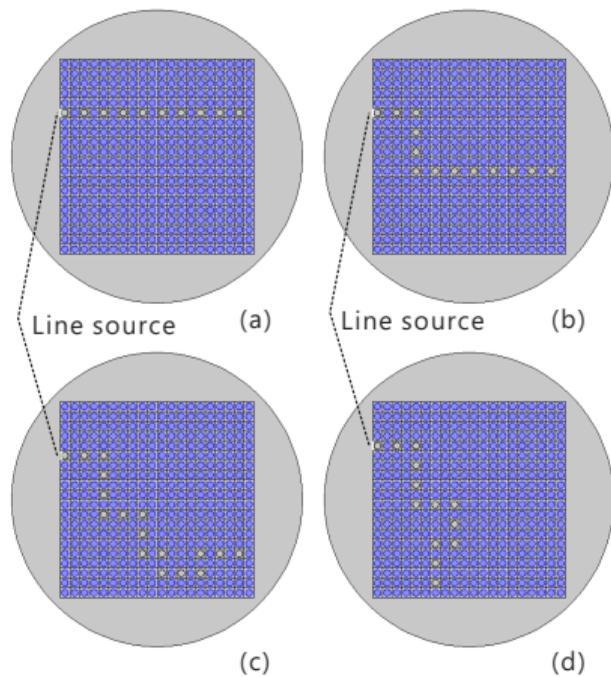
Figure: Different coupled-resonator waveguides to test the channeled spectrum idea. Square-lattice sonic crystal of mercury cylinders in water. (a)  $L = 10\Lambda$ , (b)  $L = 13\Lambda$ , (c)  $L = 17\Lambda$ , and (d)  $L = 13\Lambda$  [48].
