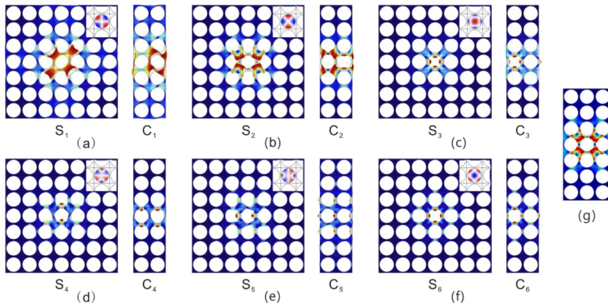
**Figure:** Displacement and pressure fields of the six defect modes of the acousto-elastic phononic crystal, shown at the  $\Gamma$  point of the first Brillouin zone.
