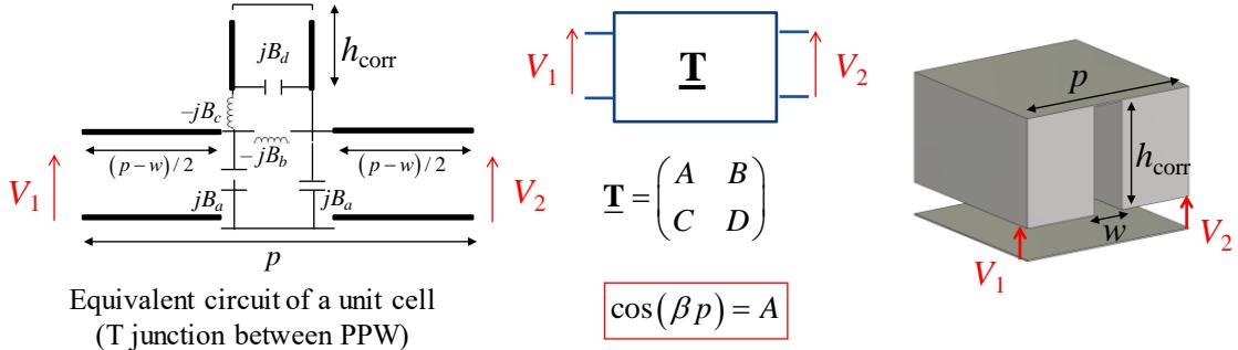
Equivalent circuit of a unit cell
