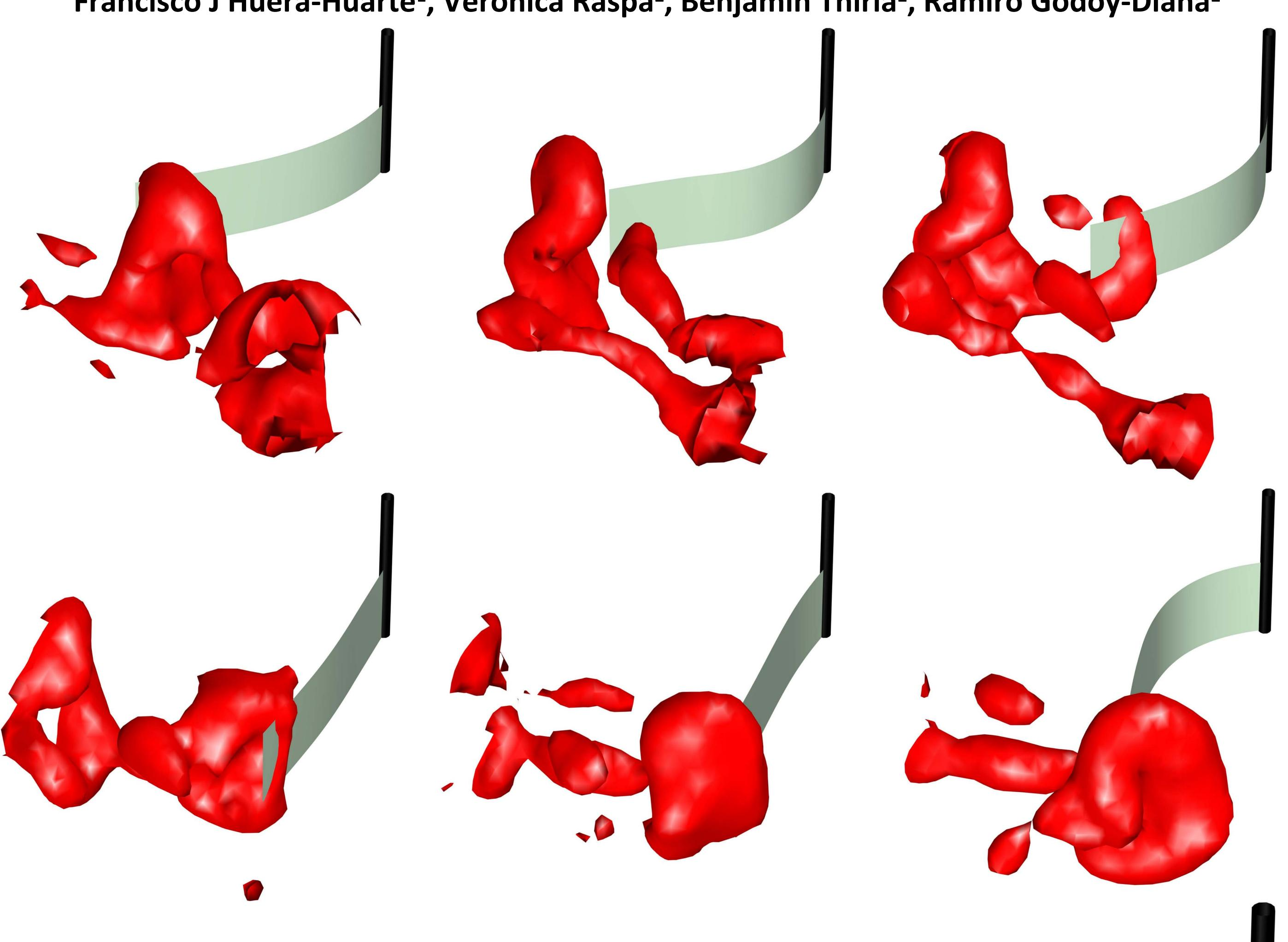
Phase averaged vorticity maps (Q-criterion) around an undulatory swimmer made of a 170 μm thick Mylar sheet of aspect ratio 0.33 (span/chord), pitching sinusoidally at the leading edge, with an amplitude of 50 degrees and a flapping frequency of 1 Hz in a still water tank.
